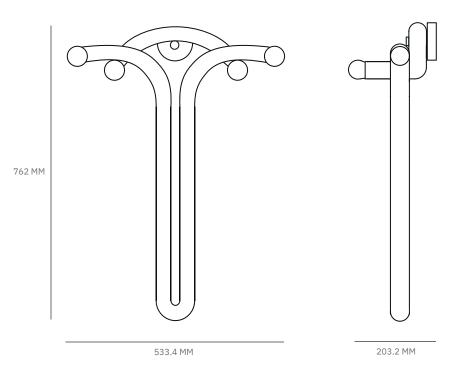
P.CODE: PMGS DIMENSIONS: 762 MM H x 533.4 MM W WEIGHT: 4 KGS LAMPING: 4 TYPE E14 SCREW BASE 3W LED, WARM WHITE - 2700K MATTE PORCELAIN FINISH CE CERTIFIED, VOLTAGE 220V - 240V DIMMABLE MATERIALS: BRASS AND PORCELAIN FINISH GLASS CUSTOM FINISHES: 1. AGED BRASS 2. BURNT BRASS 3. RAW BRASS 4. SILVERED BRASS LEAD TIME:
